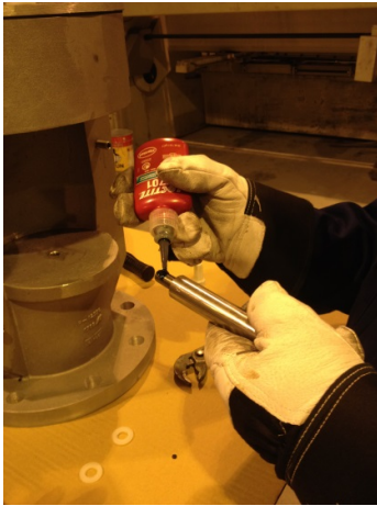
Loctite on guiding pin
