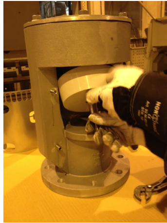
Replace floater and guiding pin
